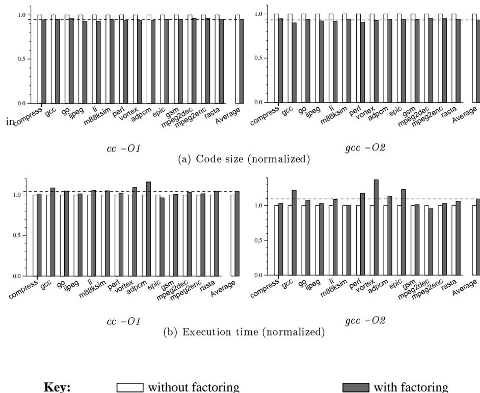
Fig. 13. Relative impact of code factoring on code size and execution time.
