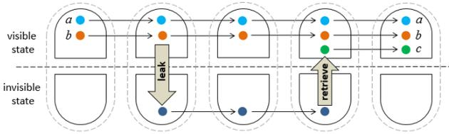
Figure 2. Information flow through visible and invisible states. The value  $a$  represents “normal” flow and occurs entirely through visible states; the value  $b$  flows through visible states, but is also injected into the invisible state and subsequently retrieved into  $c$ . The flow from  $b$  to  $c$  occurs through a covert channel.
