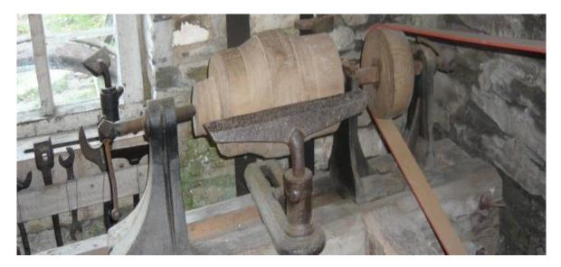
A water-driven lathe
