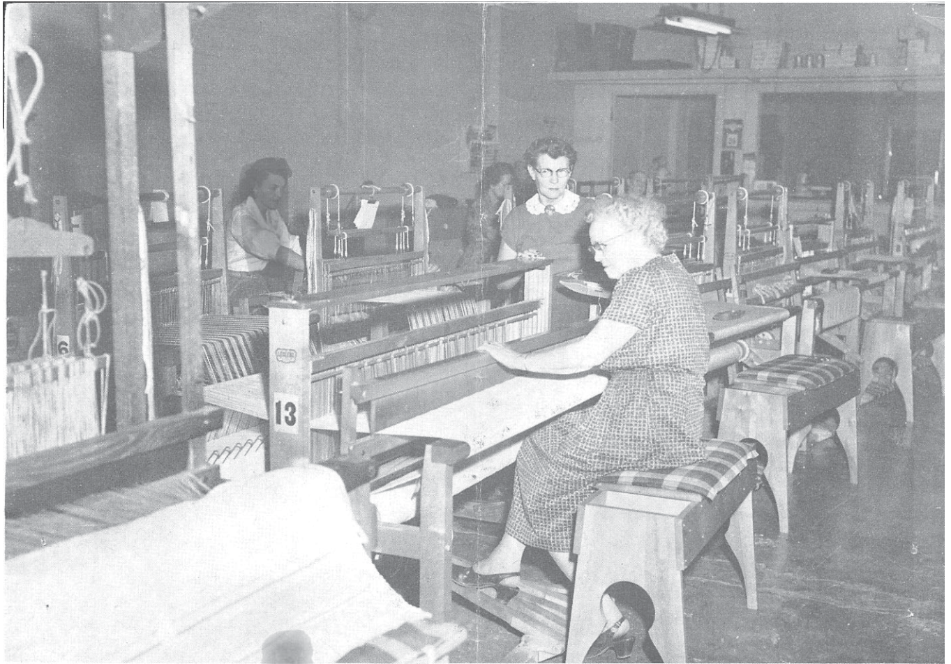
This is a view of the weaving room at the Wichita Arts and Crafts Center. Mrs. Abbie Rogers is weaving a Bronson lace table cloth with a warp and weft of 40/2 linen. The loom is a 60" Jack-type Leclerc. Mrs. McCumber, the director of the center, is watching as Mrs. Rogers weaves. The photograph was taken before classes were opened, hence the empty looms.
