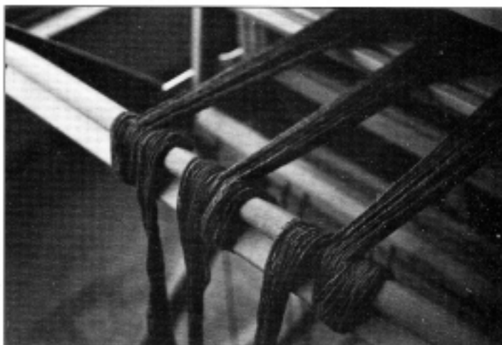
Figure 2. Warp chain wrapped around front beam to provide tension while winding on.
