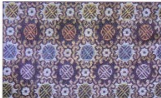
Figures 12b and 12c. Modern lampas fabric based on traditional design (possibly from the Zhuang ethnic minority), front and back side. Black background is warp-faced twill; colored pattern wefts are held on both front and back sides of the fabric by widely-spaced thin, white binding warps; the white weft of the background fabric also appears on the front of the fabric as a pattern component. (Hand woven at Nanjing Brocade Research Institute).
