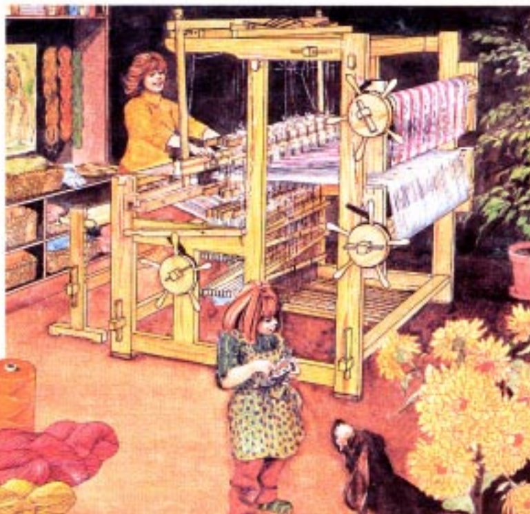
180cm (60") counter-march loom with double warp beam and fly-shuttle beater.
