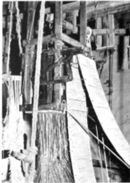
Plate 3: Detail of Jacquard mechanism on pit loom.
