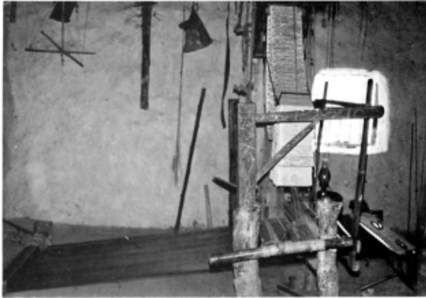
Plate 2: Jacquard pit loom for weaving sārīs . Banaras.
