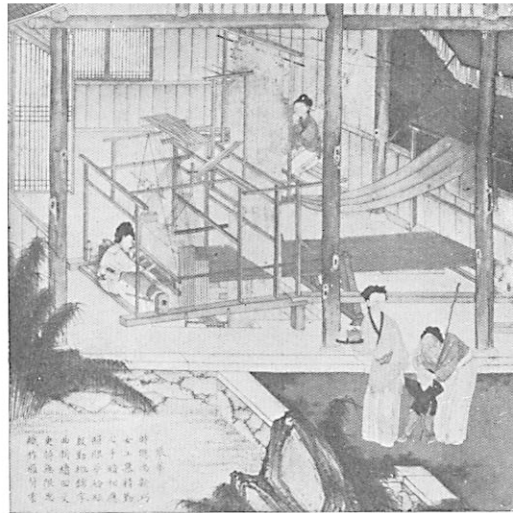
FIG. 44.—CHINESE DRAW LOOM. (From an ancient drawing.)
