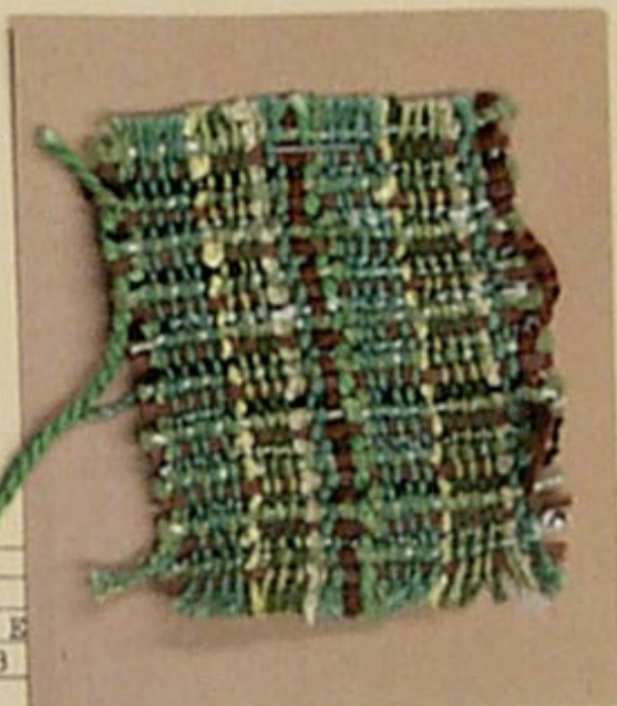
Sleyed in a 12 dent reed as below:
