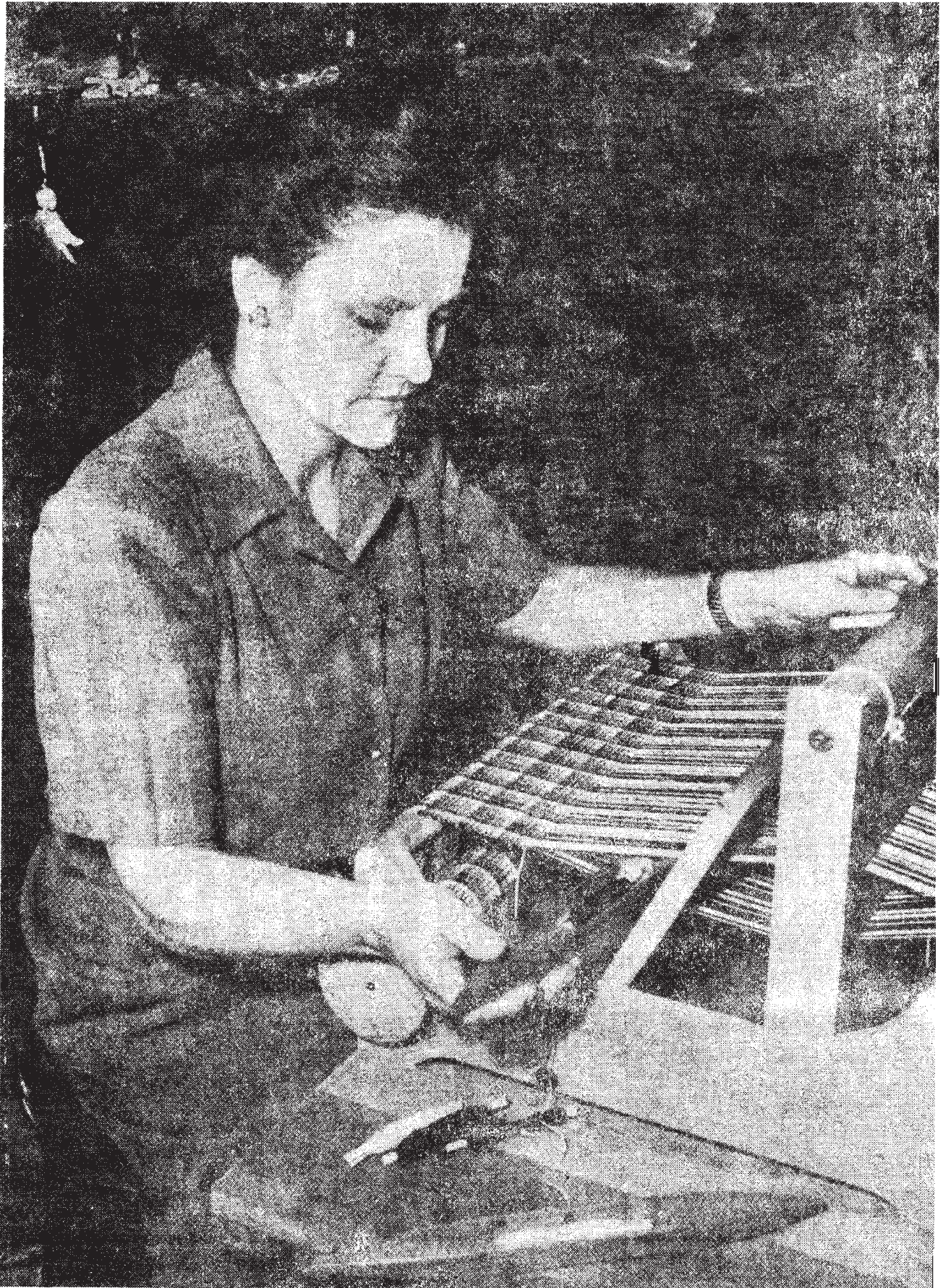
The dress is mocha nubby wool, chartreuse ratine wool, set 15 to the inch. The shirt being woven is also (x+y)^3 black, white 18/2 wool, 20 count.
