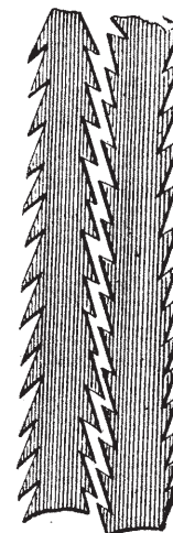
FIG. 5.—DIAGRAM TO EXPLAIN FELTING OF WOOL.
