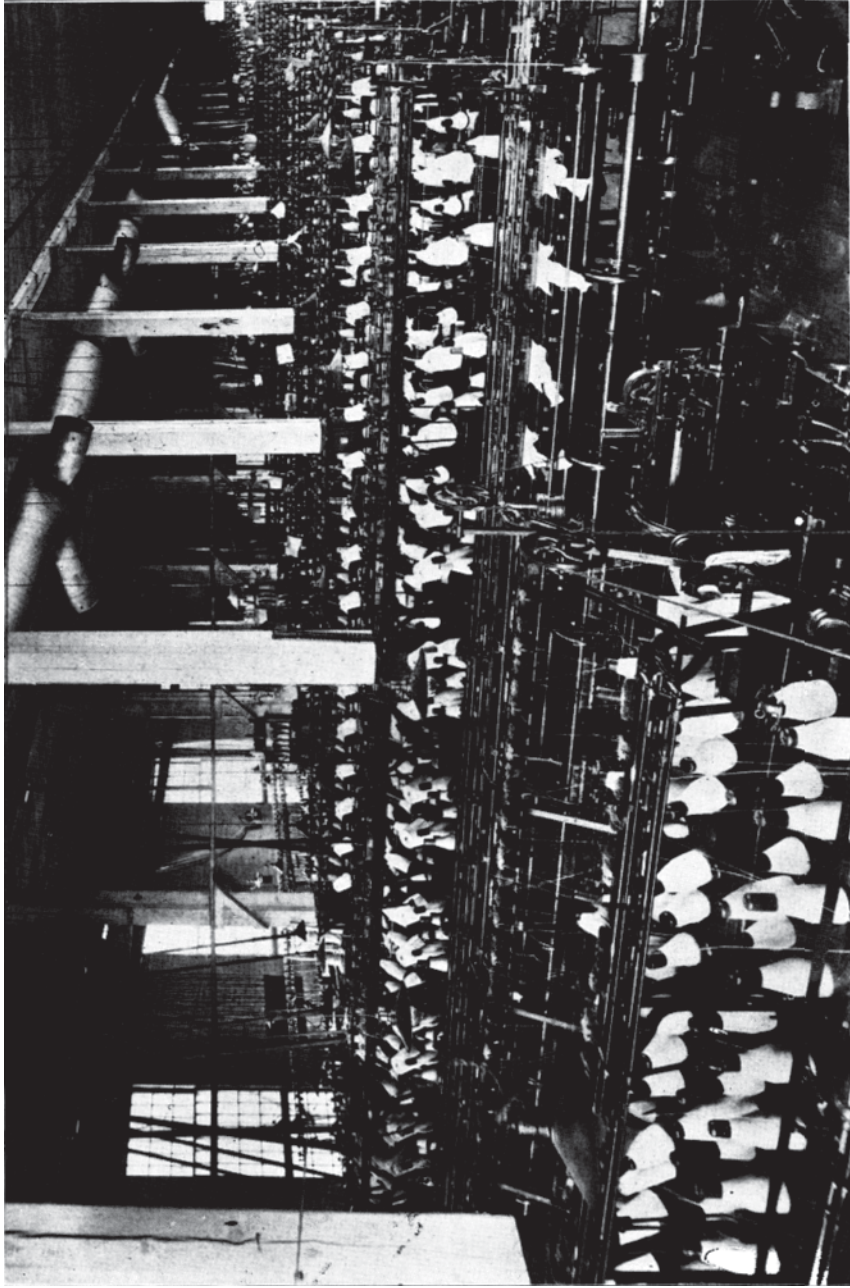
VIEW IN ONE OF THE KNITTING ROOMS AT THE WAYNE KNITTING MILLS, SHOWING 18-SECTION FOOTER AT WORK ON HALF HOSE
