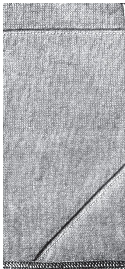
Fig. 17. "Overlock" Over-Edge for Shirts and Cuffs and "Overlock" Tailor-Made Seam for Shoulders and Gussets.
