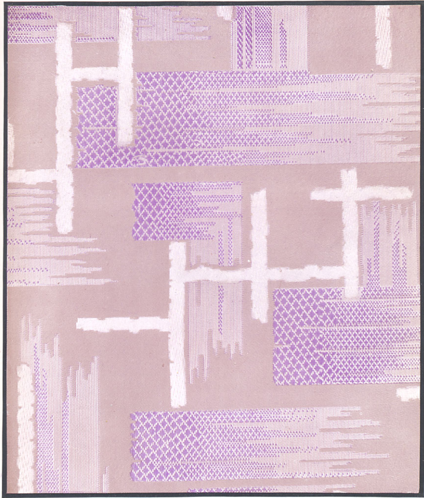
FIG. 306. SILK SPECIMEN—SHADING IN DIAMOND-WEAVE STRUCTURES.
