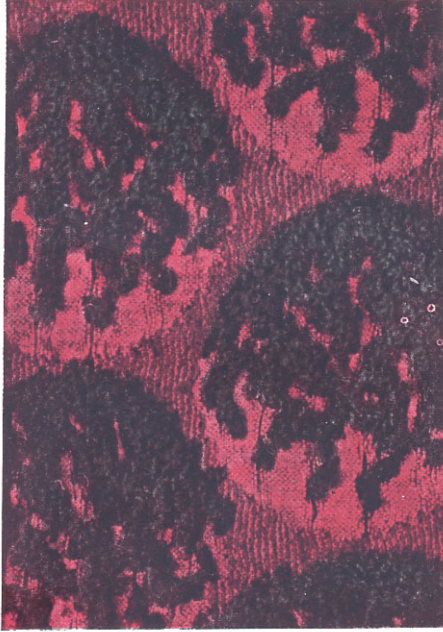
FIG. 323. SPECIMEN WITH CREPON GROUND AND TERRY-PILE SPOTTING.
