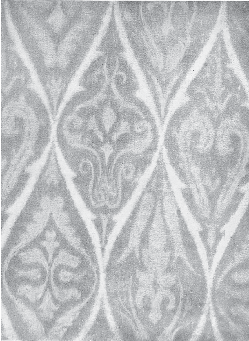
FIG. 228.—Three-ply Weft Reversible.
