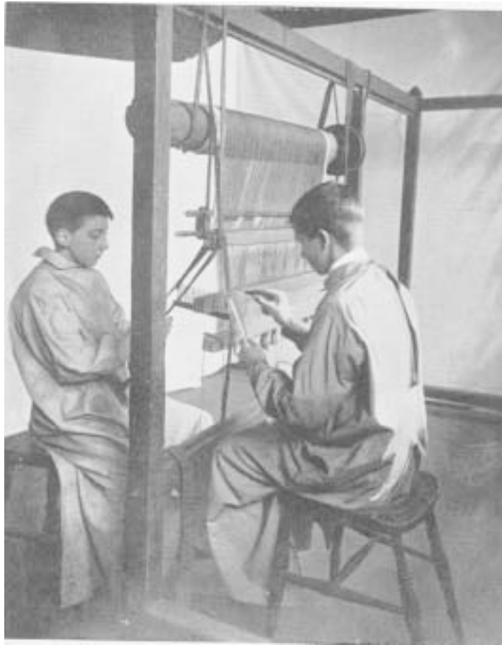
FIG. 22.—'DRAWING-IN' THE WARP
