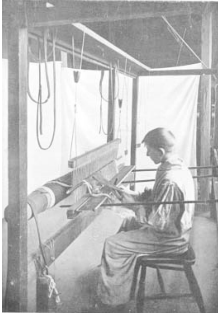
FIG. 24.—'REEDING' OR 'SLEYING' THE WARP AFTER DRAWING-IN
