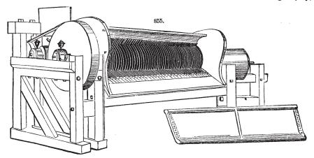
screw or bolt on which the grate-fall rests; g, back board, to which are attached the back grates and "patent moter;" h, grate-fall hollow, which is hung upon hinges, and may be raised or lowered at pleasure; i, sliding-butt, by means of which the saw-tooth may be made to assume any desired angle with the curved surface or front of the grate; j, "patent brush;" k, sliding moteboard; l, bottom board.
