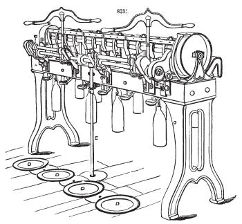
fectly equal in thickness in every part, and formed of parallel fibres; and in order to insure this, the drawing is repeated more than once, each narrow ribbon being "doubled" with others before each successive drawing.
