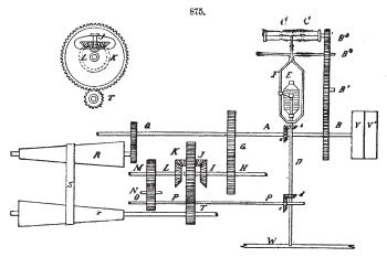
of still greater thinness and delicacy than it had before; it then gives to the roving thus produced a slight twist, sufficient to enable the fibres to cohere; and, lastly, it winds this twisted roving upon a bobbin, on which it is conveniently transferred to the spinning machine. Instead of the bobbin-
