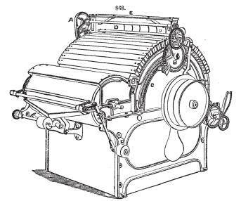
produce more perfect work: also, when the practice of sharpening is continued daily, it can be done in much less time; two men can easily sharpen 30 carding engines in the space of 4 hours. The card-belts being all fitted with buckles, no time is lost in making them long or short, for the purpose of reversing the motion of the cylinders. The tops are also brushed out and sharpened once a week.
