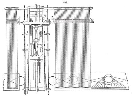
machine, we present in Figs. 883 to 886 views of the self-actor mule constructed by Mr. William Mason of Taunton, Mass. Fig. 883 is a perspective view, Fig. 884 an elevation of the opposite side, and Figs. 885 and 886 plan and elevation of carriage and drawing-rolls. This mule differs
