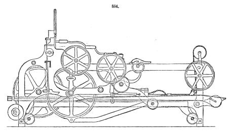
ence between the action of the throstle and the mule is, that the former has a continuous action upon the roving, drawing, twisting, and winding it upon the spindle; while the mule draws and twists at one operation as the carriage runs out, and then winds all the lengths upon the spindles as the carriage runs in.\*
