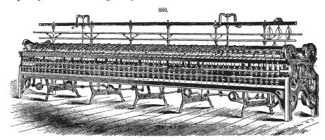
yarn, now goes to the spinning-machine, which may be a throstle or mule; the ring-throstle being generally used in the United States for warp, and the mule for weft, though either machine is occasionally employed for both purposes. Fig. 880 shows the ring spinning-frame of the latest pattern, as built by the Whitin Machine Company.
