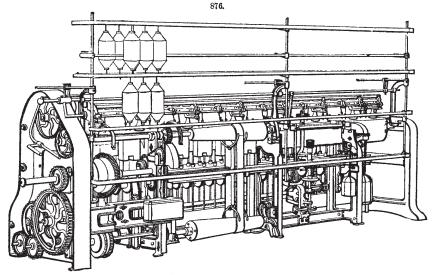
the roving to the proper size for the yarn to be produced, doubling the roving to insure greater evenness before drawing at each operation.
