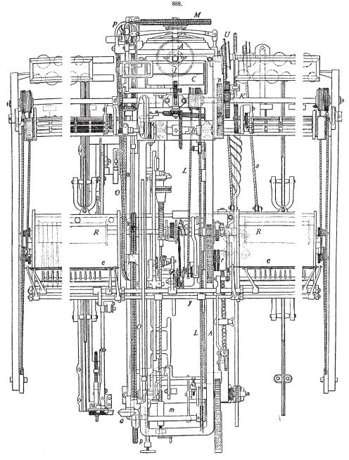
leys C, and, through another bevel-gear, gives motion to the winding-scroll U, Fig. 887, around which the band e passes through the carriage, and is made fast to a take-up ratchet on the front side, and draws in the carriage to the roller-beam, when the stretch and twist are completed. When the belt is on one of the pulleys C, the carriage is drawn out, and the rollers are put in revolution, by the shafts B and K, driven by the rim-shaft I; and when the stretch is completed, a spring
