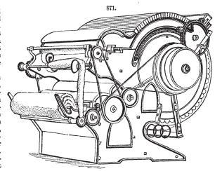
IV. Drawing-Frames.—The cotton leaves the carding engine in the state of a delicate, flat, narrow strip or ribbon, called a sliver; and these slivers have now to be converted into drawings by being elongated, narrowed, and thinned to a still more delicate condition. In the first place the slivers are collected in tall cans, from two to six in number, on one side of the "drawing-frame," and are from thence carried upward to two or more pairs of rollers, the two rollers of each pair revolving
