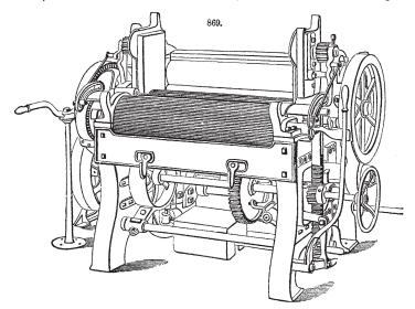
of the finisher-card, to which they are transferred. This lap-head is shown in perspective in the The cards for this would usually be arranged in 4 or 6 sections of 16 each, according to the width of the mill, and placed longitudinally in the same; while at the end of each section a belt running transversely would receive the slivers from that section, uniting in one broad sheet at the lap-head, which would stand in line with the last section.
