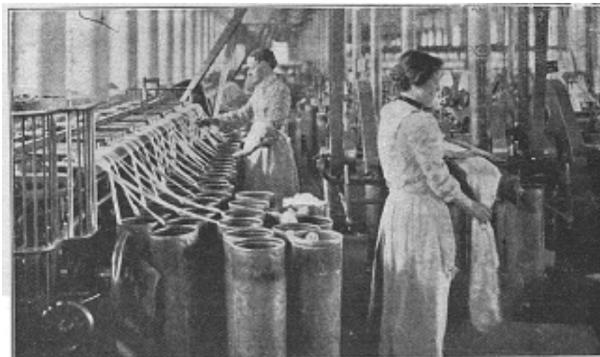
DRAWING SILK PREPARATORY TO SPINNING
