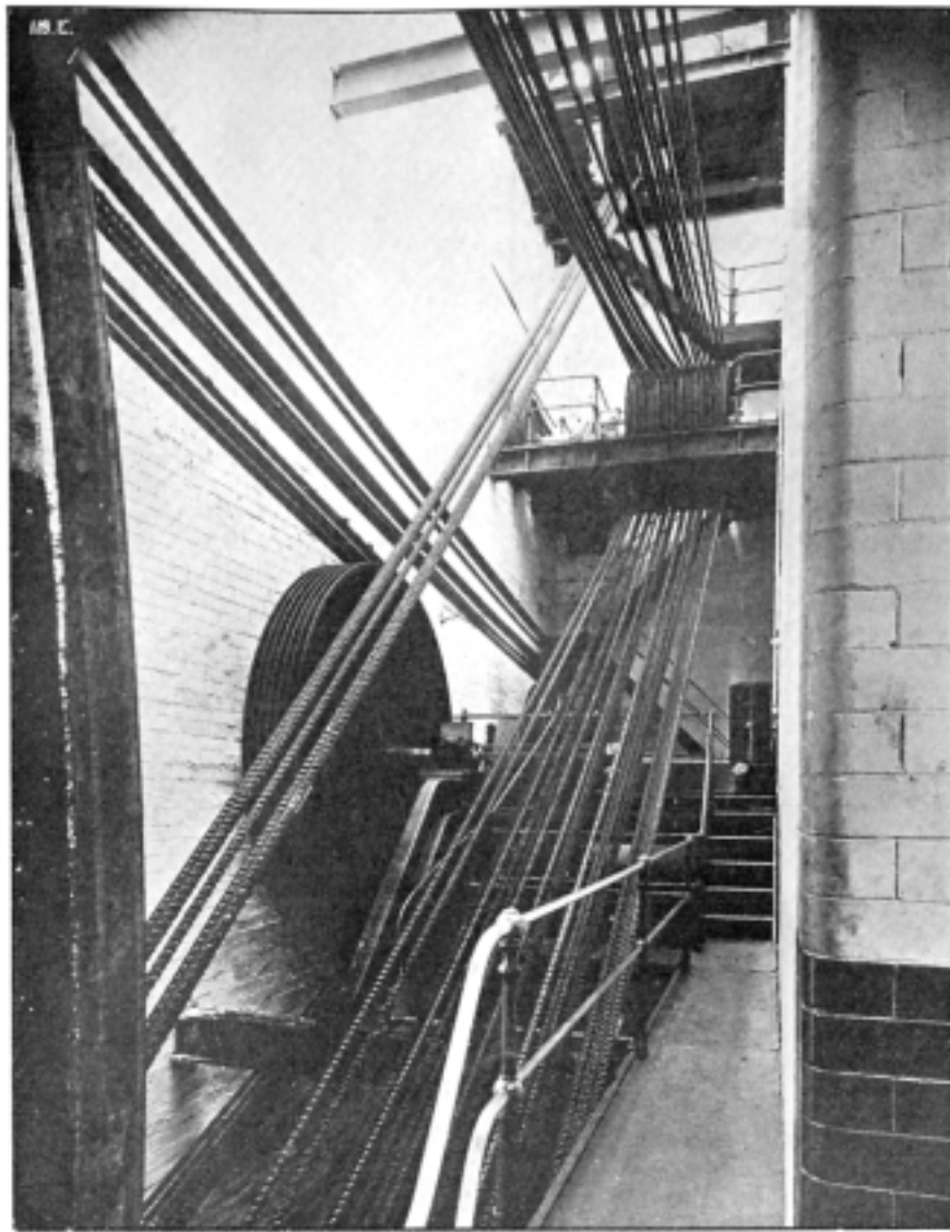
FIG. 2.—VIEW SHOWING TRANSMISSION ROPE-RACE USED IN CONNECTION WITH ENGINE SHOWN IN FIG. 1. MESSRS. HICK, HARGREAVES & CO., LTD., BOLTON
