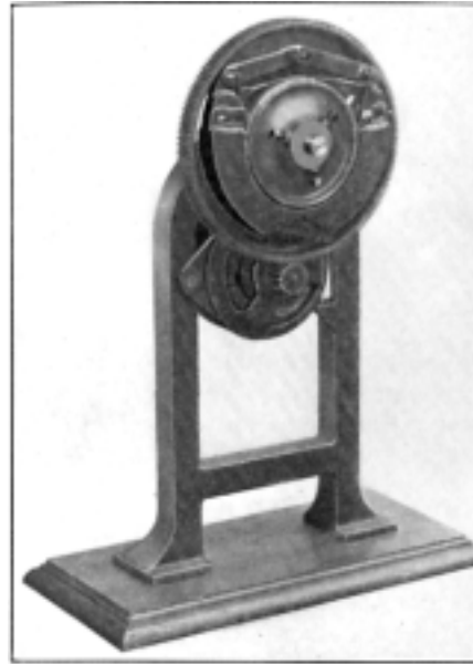
FIG. 7.—CENTRIFUGAL DEVICE TO PERMIT MOTORS RUNNING UP NEARLY TO FULL SPEED BEFORE THE LOOM IS STARTED. MESSRS. SIEMENS BROS., LTD.
