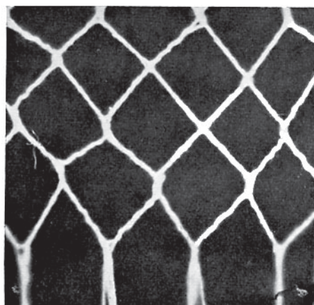
NO. VII.—RÉSEAU OF LUCENA, PUNTO DE AGUJA, RECONSTRUCTED UNDER THE MICROSCOPE BY E. M. W. THE DOUBLE THREAD IS TWISTED FIVE TIMES, OCCASIONAL ERRORS OCCURRING IN THE TWIST
