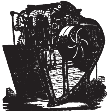
Rotary Fulling Mill. (Top casing removed.)
